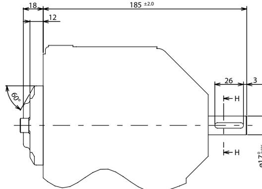
Pump Shaft : 17mm Straight Keyed (Key Length 36mm)
