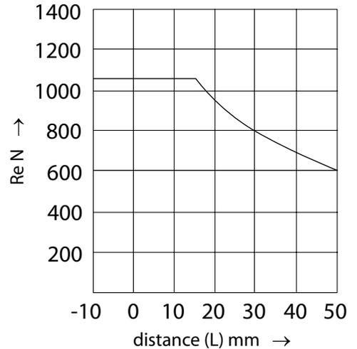
The maximum shaft thrust in ( $T_{in}$ ) of input shaft is 18% of allowable radial load ( $Re$ ) of the input shaft.
