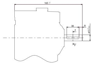
Pump Shaft : 15mm Straight Keyed PTO Shaft : None
