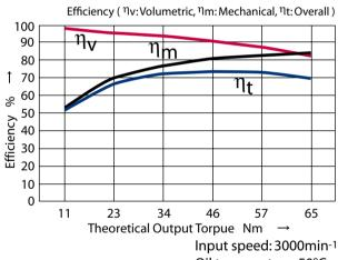
Input speed: 3000min Oil temperature: 50°C Full Displacement
