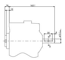
Pump Shaft : 15mm Straight Keyed PTO Shaft : None
