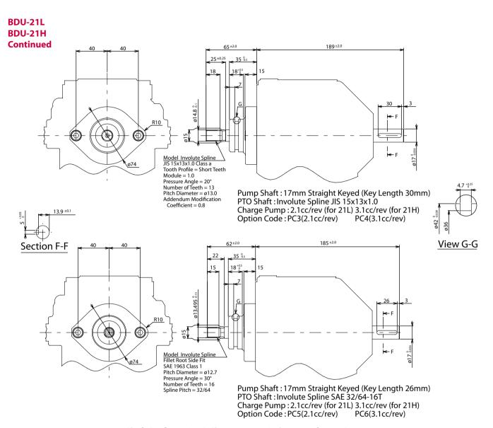
Shaft Configuration & Charge Pump Displacement for 21L & 21H
