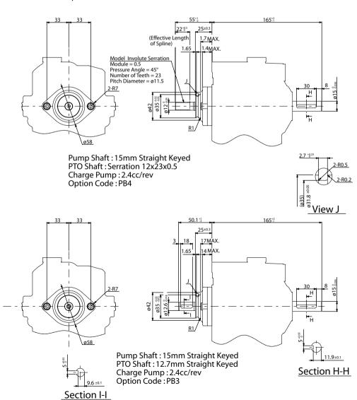
Shaft Configuration & Charge Pump Displacement for 10L
