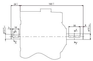
Pump Shaft: 15mm Straight Keyed PTO Shaft: 12.7mm Straight Keyed Charge Pump: None
