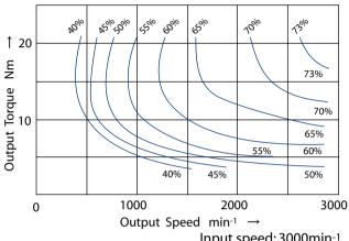
Input speed: 3000min-1 Oil temperature: 50°C
