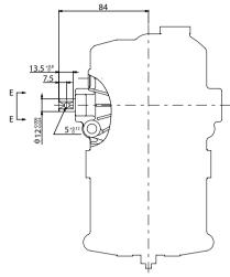
Left-hand side viewing from input shaft (when pump located upside) Option Code: L
