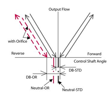
Input speed: 3000min-1 Oil Temp: 50°C
