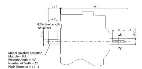
Pump Shaft: 15mm Straight Keyed PTO Shaft: Serration 12x23x0.5
