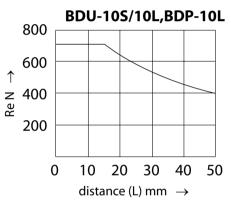
The maximum shaft thrust in (**Tin**) of input shaft is 18% of allowable radial road (**Re**) of the input shaft.
