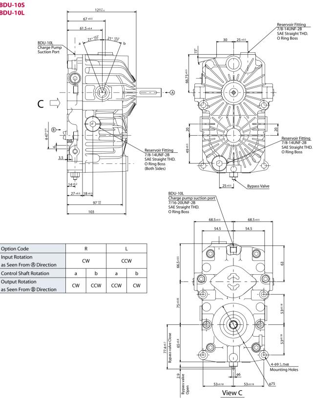
NOTICE: The tightening torque to install HST is 1569 to 2058 N·cm.
