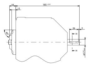
Pump Shaft: 17mm Straight Keyed (Key Length 36mm)
