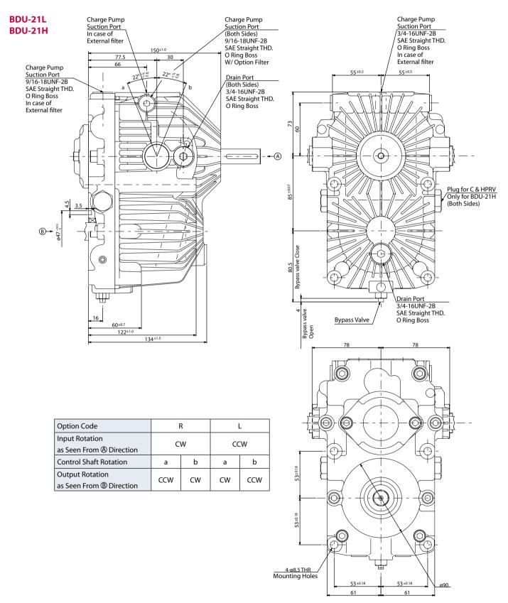
NOTICE: The tightening torque to install HST is 1569 to 2058 N⋅cm.
